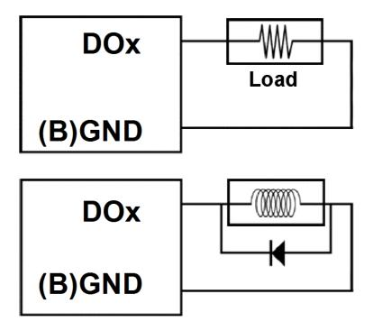
**Note:** while connect inductive load (drive relay), the diode is needed for prevent the counter EMF.
