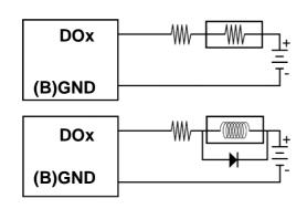
**Note:** while connect inductive load (drive relay), the diode is needed for prevent the counter EMF.
